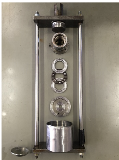
Fig4.2 Insertion order of oil tank and thrust ball bearing
