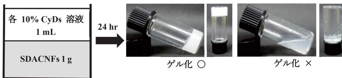
Fig. 16. Preparation of SDACNFs/cyclodextrins gel.
